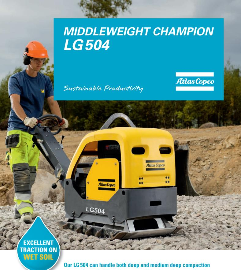
Our LG 504 can handle both deep and medium deep compaction of granular soils. Like all our reversible plates, it is an effective alternative and complement to rollers when compacting soil in confined areas.
