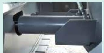
**Crawler extension/retraction mechanism guard**
