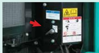
**Battery shut-off device**
