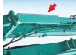
Guided reinforced bucket cylinder guard with box-type structure
