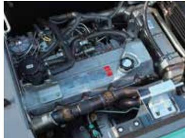
A new electronically controlled engine with high power and low fuel consumption is installed. Particulate matter and NOx emissions are suppressed through the engine's high combustion efficiency, exhaust gas after-treatment equipment, and urea SCR system. The engine also conforms to EPA Tier IV Final regulations.
